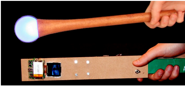
Figure 7. Both ‘Magic Wand’ prototypes. (a) the shape model (top); the technical model (bottom).
