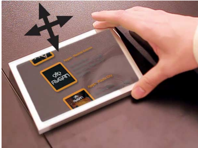
Figure 4. Exploring a list of songs by moving the phone on a table.
