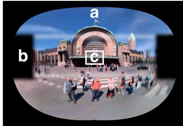
Figure 2. A fisheye representation of the user's field of view: a) the binocular visual field, b) the Epson glasses' frames, and c) the virtual image of the HMD at 23 degrees diagonally, covering only \sim 1/10 of the horizontal binocular visual field.
