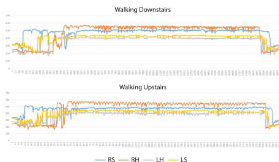
Figure 2: Sensor readings comparing walking upstairs and walking downstairs (RS – Right Shoulder, RH – Right Hip, LH – Left Hip, LS – Left Shoulder)
