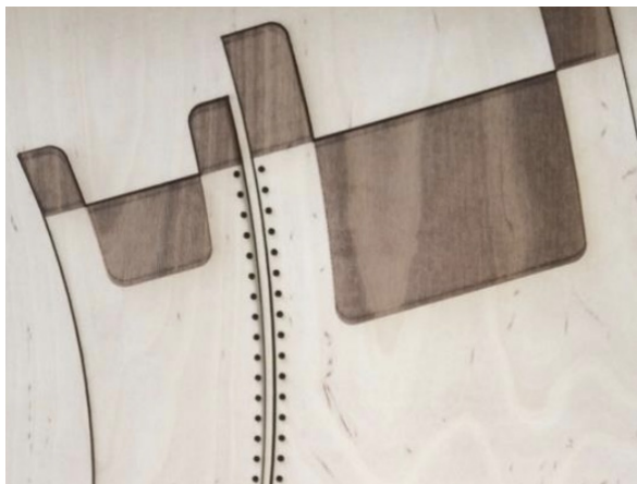
Figure 2: Laser cutting and engraving process
