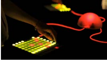
Figure 1: PolyMetros create musical sequence from each pad and result will combined on the center hardware.
