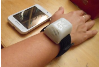
Figure 1. ABBI bracelet together with a mobile device. By default the ABBI is quiet when it is stationary, and only makes sounds when it is moved.
